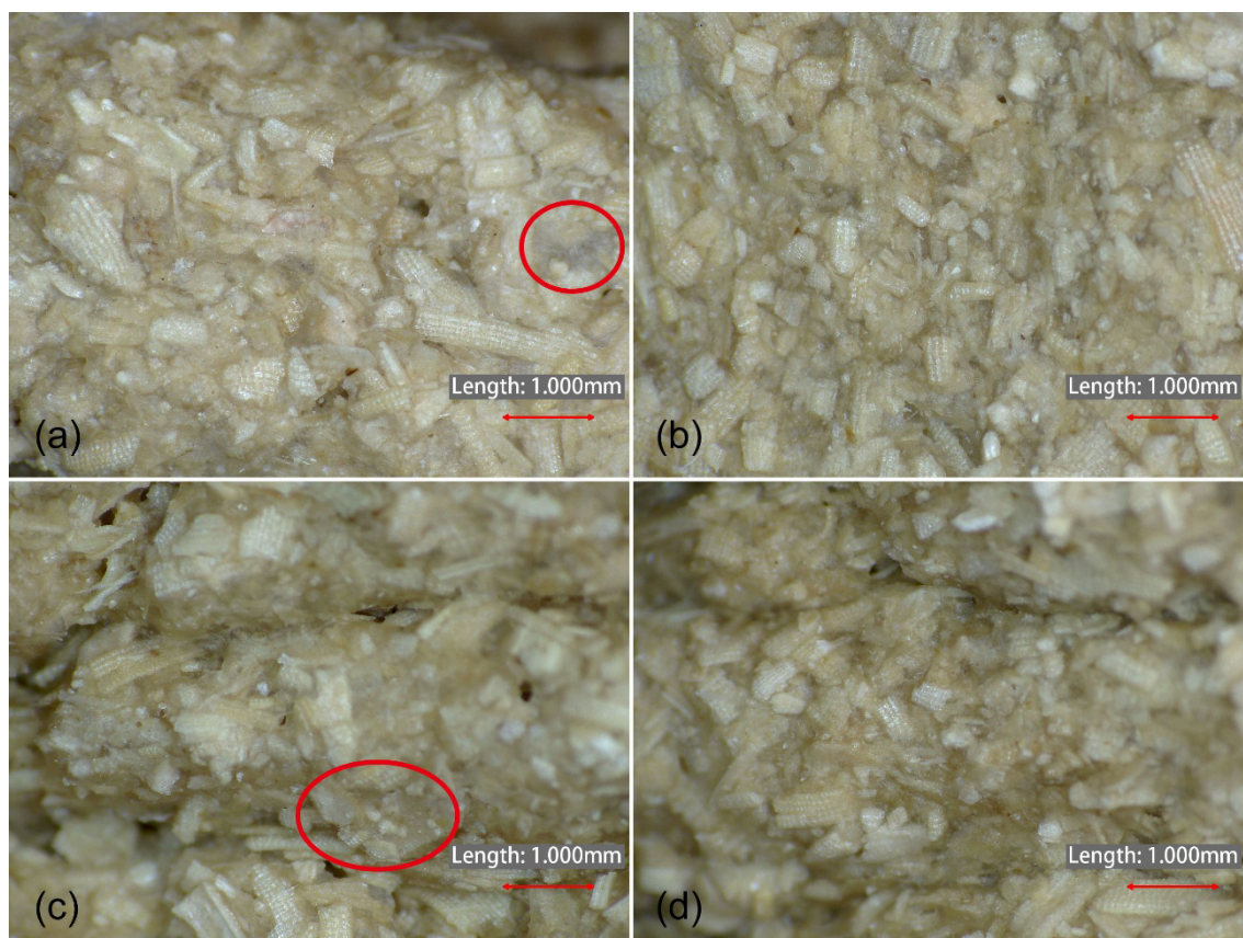
Fig. 14 Magnified images of 3D printed objects using rice husk paste (a) crushed rise husks: top (b) rice husk powder: top (c) crushed rise husks: side (d) rice husk powder: side.
