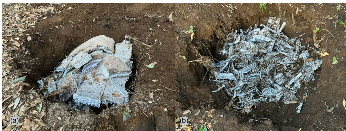
Fig. 10 Testing for unit disassembly. (a) The small-scaled temporary structure was successfully dismantled into units (October 14, 2023). (b) After being buried in the soil for one year (October 14, 2024).
