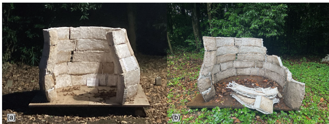
Fig. 9 Progress observation (a) Initial relocation (November 15, 2022). (b) Partial damage occurred at the joint (August 6, 2023).
