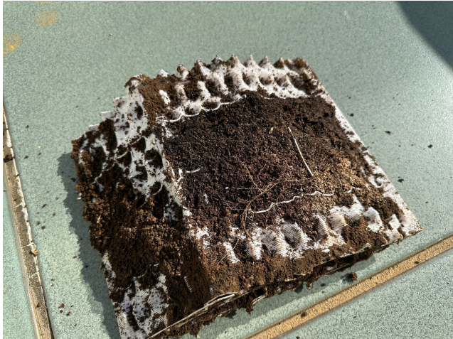
Fig. 11 Unit buried for 365 days. The mycelium-based composite had disappeared.
