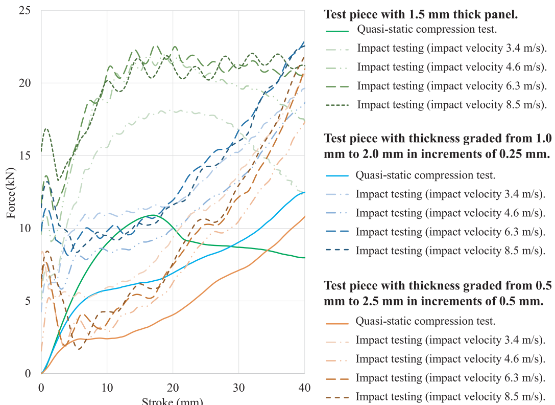
Fig. 10 Force-stroke curves of test pieces.
