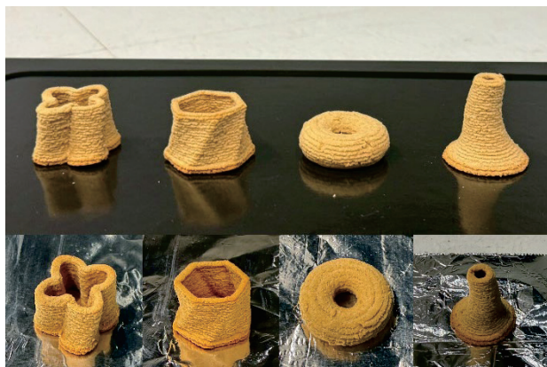
Fig. 4. Actual Printing Results of Food Shapes with Various Geometric Structures
