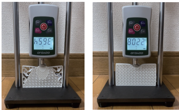
Fig.5. Compression test setup: (a) Streccs3D-applied infill, (b) uniform infill
