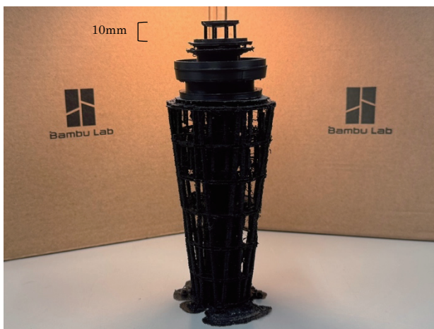
Fig.6 3D model of Enoshima Sea Candle derived from 3D point cloud data obtained via handheld LiDAR scanning
