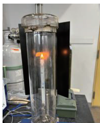
Fig.4. Measuring apparatus for Limiting Oxygen Index
