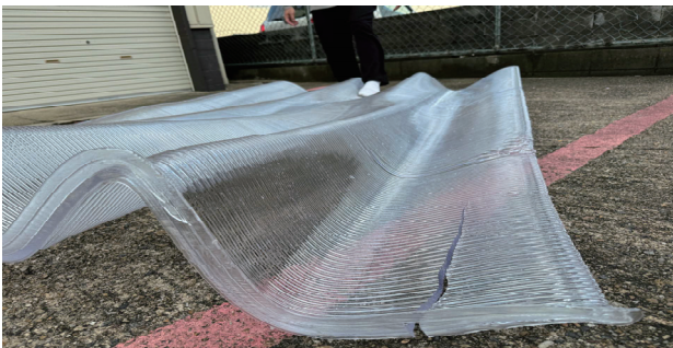
Fig. 2. Cracking due to residual stress and layer misalignment
