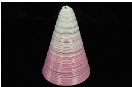
Fig.9 Egg pack recycled material Mini traffic cone
