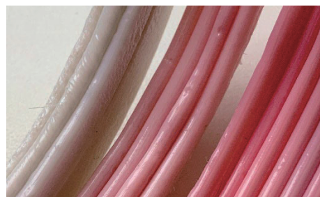
Fig.7 Egg pack recycling material output sample
