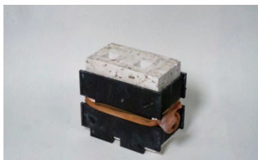
Fig.6. Slip casting in progress
