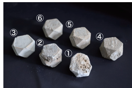
Fig.4 6 samples placed outdoors for 3 weeks
