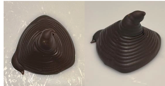
Fig. 4. The printing result at 35^{\circ}\text{C}
