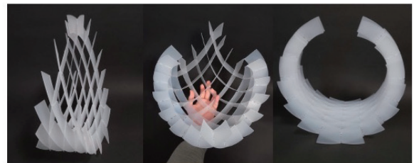
Fig. 2. Deployment behavior of a radial-slit sliceform with arc-shaped elements
