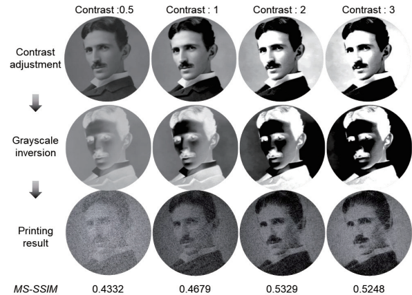
Fig.5. Printed results with different contrast of the original image. All patterns were generated with 300 nodes and 4000 fibers
