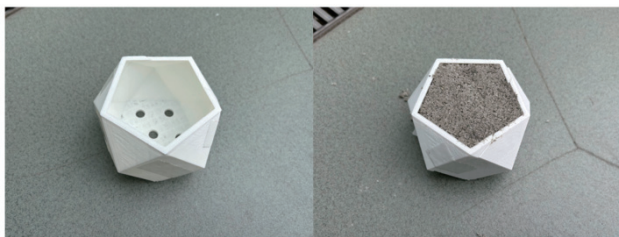
Fig.5 Formwork made with a 3D printer
