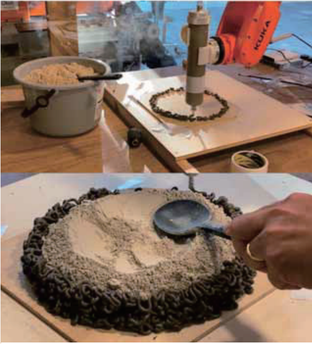
Fig. 3. Printing workflow utilizing powder-based molds
