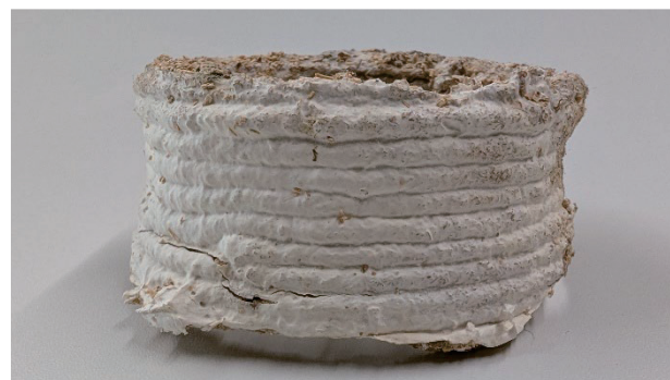
Fig. 6. Rice husk structure coated with oyster mushroom fungus
