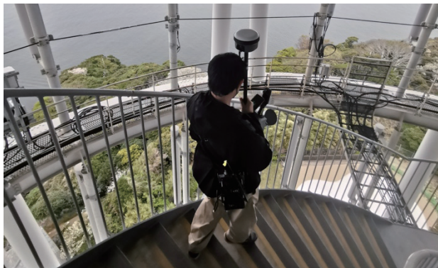
Fig.2 Photograph showing the measurement process of 3D scanning using a handheld LiDAR and RTK-GNSS
