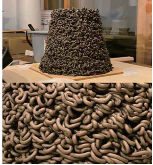
Fig. 4. The 'organized chaos' structure of the 3D printed clay
