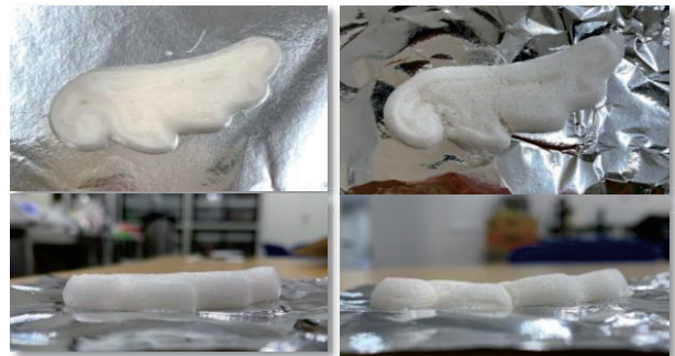
Fig. 3. Changes in foam-shaped objects over time (left: immediately after printing, right: 10 days later)
