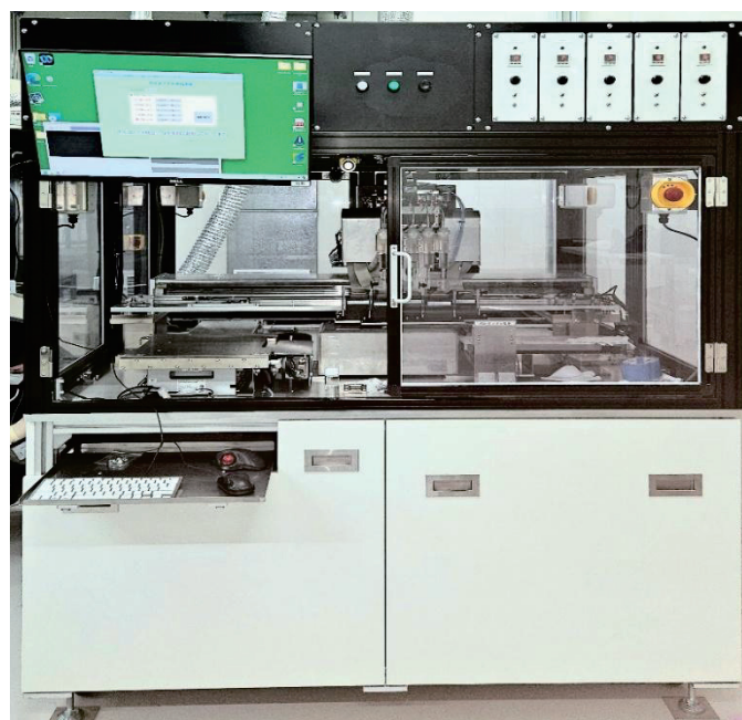
Fig10. 300 mm coating machine for perovskite solar cells.
