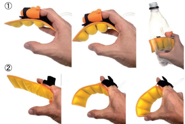
Fig. 6. Augmented finger actuator
