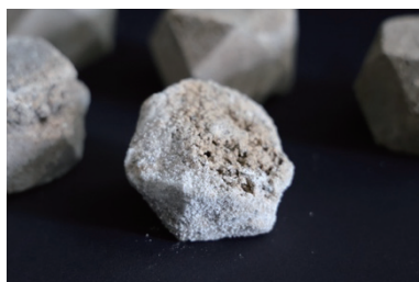
Fig.6 Sample① with pronounced efflorescence
