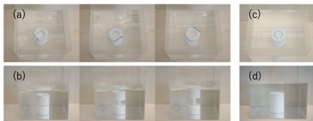
Fig.11. Underwater deformation of combined device: top-floating (a)(b), bottom-floating (c)(d)
