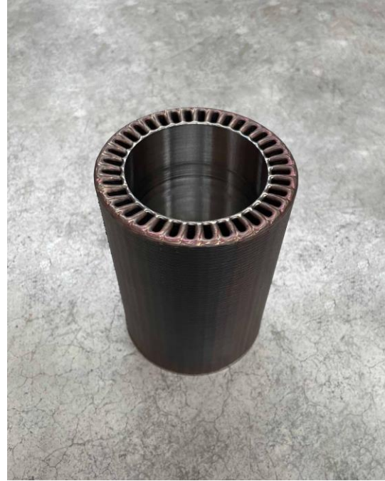
SS316L +Inc718 – Dual Material Pipe Meltio M450 Size: \Phi 108.0 x 150.0 mm Weight: 5 kg Print Time: 12 h 原材料費: 38,000円
