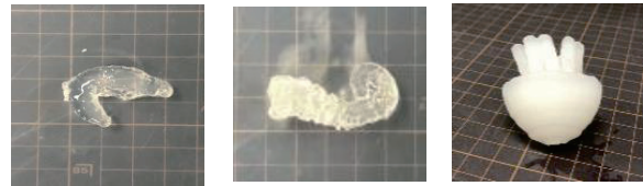
Fig. 2 Food formed samples by RepRap SWIM-ER (Prawn, Octopus leg, Jellyfish)
