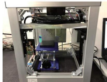
Fig. 1 Gel 3D Printer “RepRap SWIM-ER”
